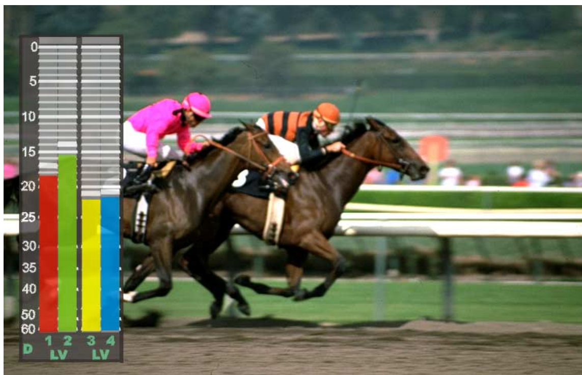
The E-Series bargraph (full size AES/EBU scale) mixed against video background
